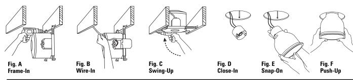
WARNING: USE ONLY WITH LIGHTOLIER REFLECTOR TRIMS MARKED WITH I.C. LAMPING INFORMATION. USE OF OTHER MANUFACTURERS' TRIMS VOIDS THE UNDERWRITERS LABORATORIES LISTING AND COULD CONSTITUTE A FIRE HAZARD
